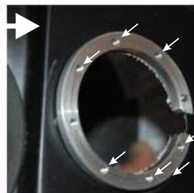
Remove Base Ring again and place reinforcement ring on the outside of the helmet. This helps to mark the exact positions for the 3mm screws. Mark only 2 opposite holes for the moment. Make sure you mark exact positions.
