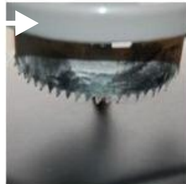
Drill with a 51mm drillsaw through the same point.
