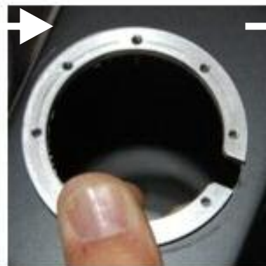
Remove Base Ring again and place reinforcement ring on the outside of the helmet. This helps to mark the exact positions for the 3mm screws. Mark only 2 opposite holes for the moment. Make sure you mark exact positions.
